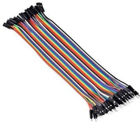
Figure 4: Male-female jumper wires
